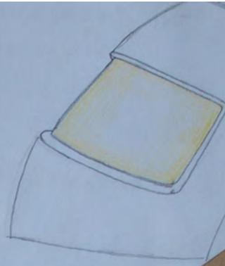
L.E.D strip being inside the casing creates a 'glow' due to the casing creating a soft shield to the surroundings
