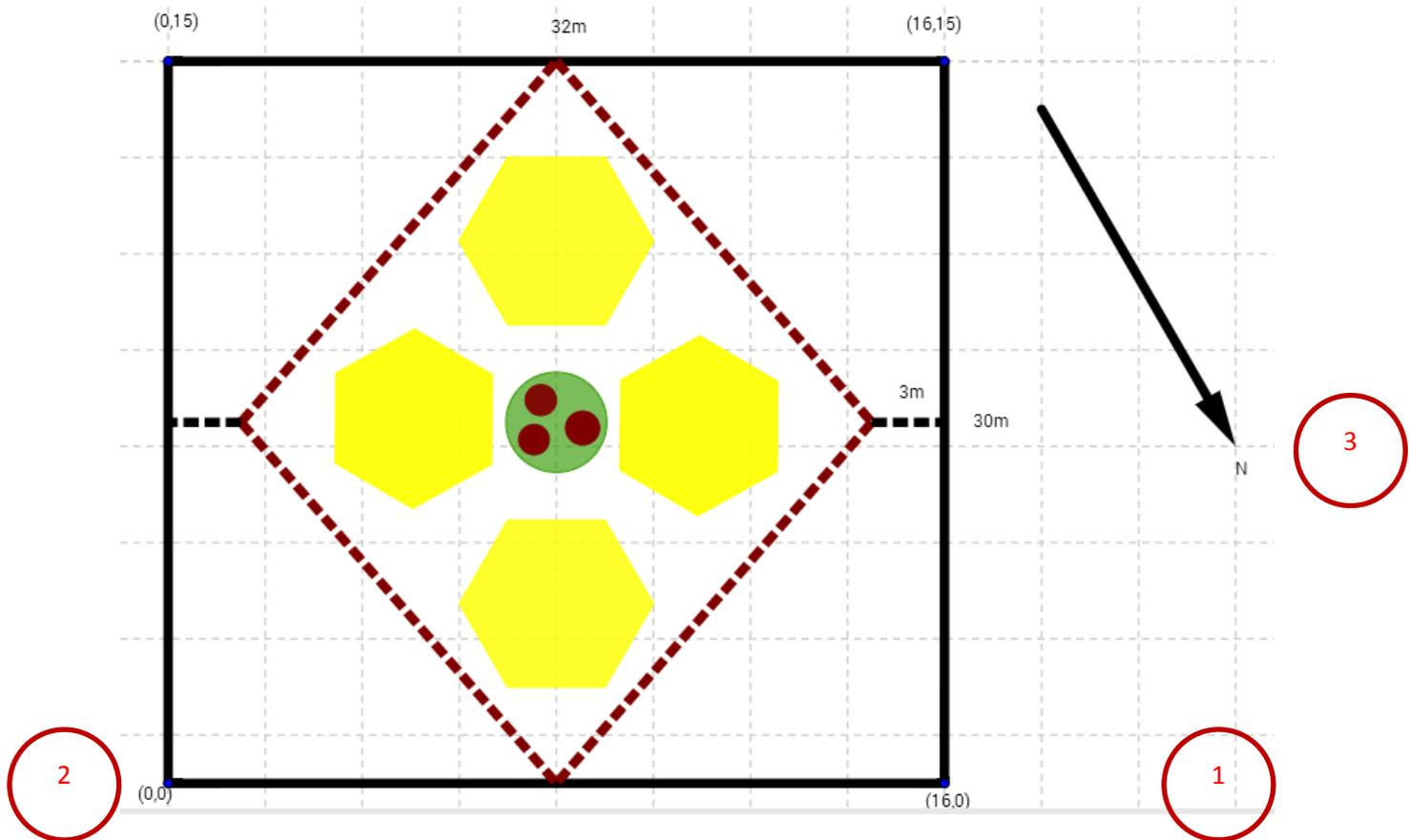
The scale of the plan is 1:200 so 1 cm on the plan is 2m on the ground. Each square on my graph paper is 2cm.
