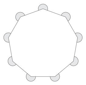
The "edge angles" of the nonagon are the angles on the outside of each vertex. They are shaded in grey on the diagram.
