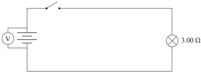
The battery voltage is measured to be  $6.02\ \text{V}$  when the switch is open. However, when the switch is closed, Casey notices that the battery voltage drops to  $5.85\ \text{V}$ .
