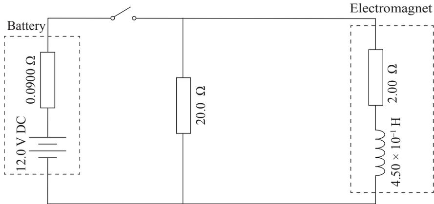
At one point, shortly after the switch is closed, the rising current drawn from the battery has reached  $2.00\ \text{A}$  and a back EMF of  $9.00\ \text{V}$  has been induced across the inductor.
