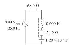
Explain why the voltage across the  $68.0~\Omega$  resistor reaches a maximum value at one particular frequency.
