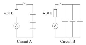
For each circuit, explain how the current varies over time compared to the single capacitor in series with a 6.00  $\Omega$  resistor, as in part (c).
