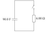
(i) Sketch a graph of current against time for 2500 s after the switch is closed.
