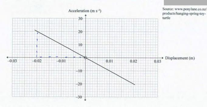
Given the equation relating to simple harmonic motion as  $a = -\omega^2 y$ , describe how the gradient of (a) the graph line relates to the frequency of oscillation.
