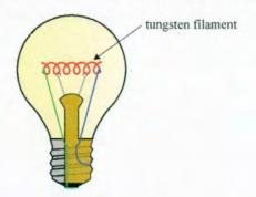
Tungsten is a metal with a very high melting point and a relatively small specific heat capacity. The very small diameter of the filament means that the filament has a large resistance.
