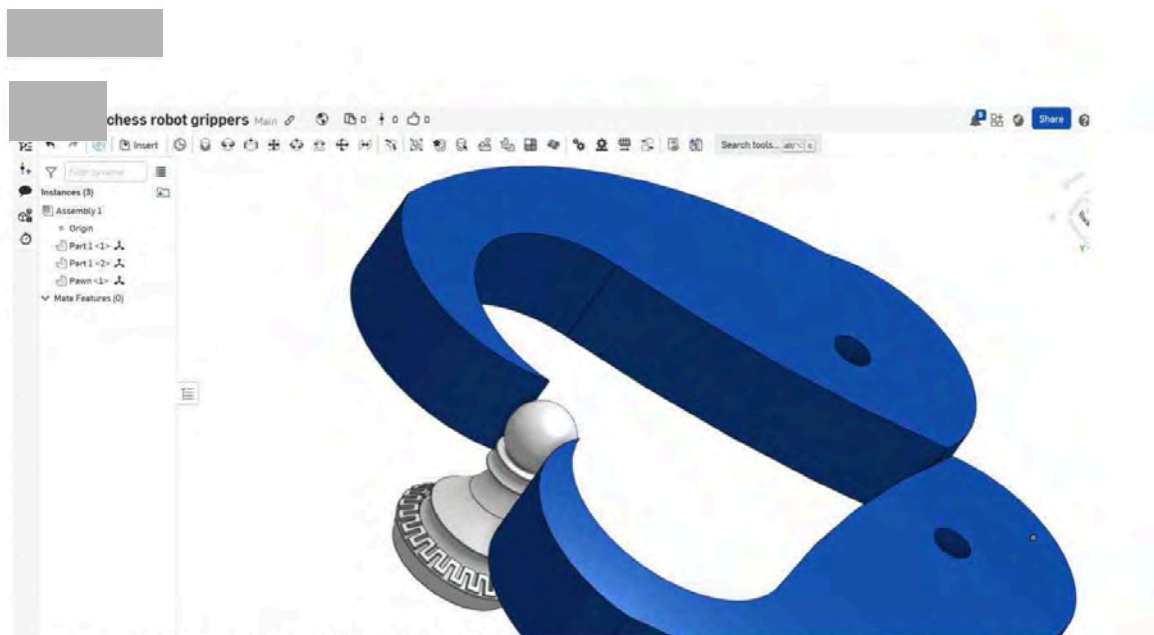
Figure 4: This is an image of be 3D modelling and simulating the claw grippers. I saw that the contact between the gripper and the chess pawn was small, making the pawn easy to slip out.
