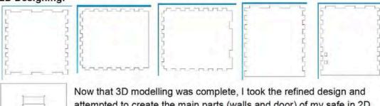
Now that 3D modelling was complete, I took the refined design and attempted to create the main parts (walls and door) of my safe in 2D using 2D Design, a 2D modelling software. Because most key factors were resolved throughout 3D modelling, this process was quite simple and straightforward.
